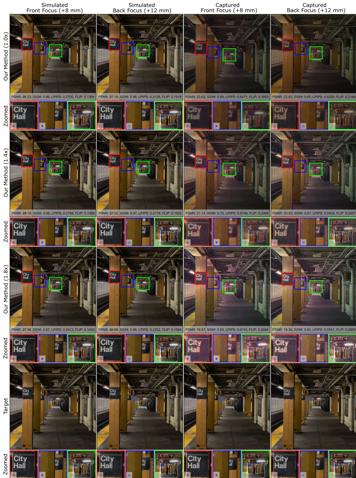
Fig. 28. The simulated and captured short Z distance reconstructions comparison of student model (RGB-only) when peak brightnesses are 1.0, 1.4, and 1.8. The volume depth of the results is 4 mm and the propagation distance is 2 mm. The resolution of the tested hologram is 2816 × 2816. All the photographs are captured at 16.6 ms exposure time (Source Image: [65]).
