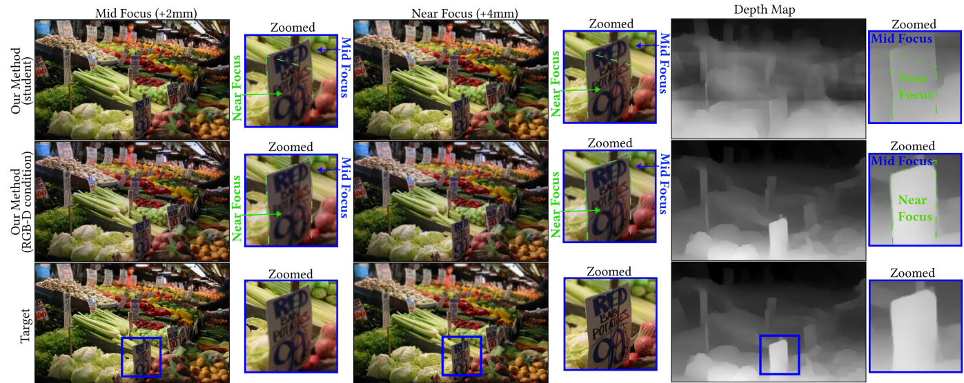
Fig. 20. Depth estimation errors causing incorrect defocus in high-resolution images. The student model predicts the top of the price board at the mid-focus plane, leading to erroneous reconstructions in the mid- and near-focus planes. Blue indicates the mid-focus region and green the near-focus region. (Source image: [88]).
