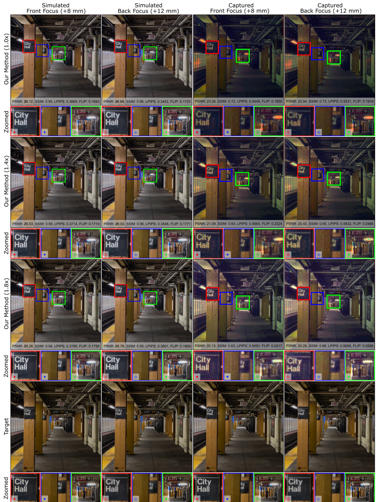
Fig. 29. The simulated and captured long Z distance reconstructions comparison of student model (RGB-only) when peak brightnesses are 1.0, 1.4, and 1.8. The volume depth of the results is 4 mm and the propagation distance is 10 mm. The resolution of the tested hologram is 2816 \times 2816 . All the photographs are captured at 16.6 ms exposure time (Source Image: [65]).
